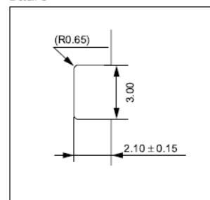
(All dimensions are in millimeters with ±0.15mm tolerance unless specified otherwise.)
