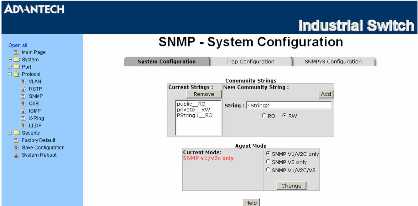
Figure 3.3-37 SNMP System Configuration interface
