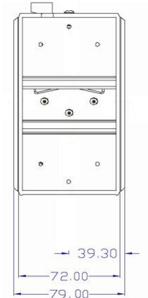
Figure 2.2-3 Rear View of EKI-7554MI/SI
