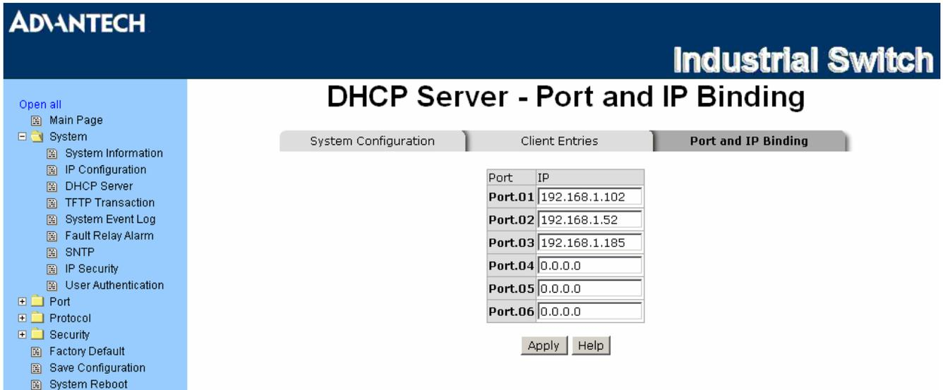
The screenshot shows the ADANTECH Industrial Switch web interface. The main title is "DHCP Server - Port and IP Binding". There are three tabs: "System Configuration", "Client Entries", and "Port and IP Binding". The "Port and IP Binding" tab is selected. Below the tabs is a table with two columns: "Port" and "IP".
