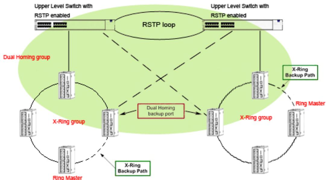
*Note* The Ethernet switches with firmware version before v3.0 use the **X-Ring** function that has the limitations as follows. However, the ones with firmware version after v3.0 (included) use the **X-Ring Pro** function that gets rid of the limitations.
