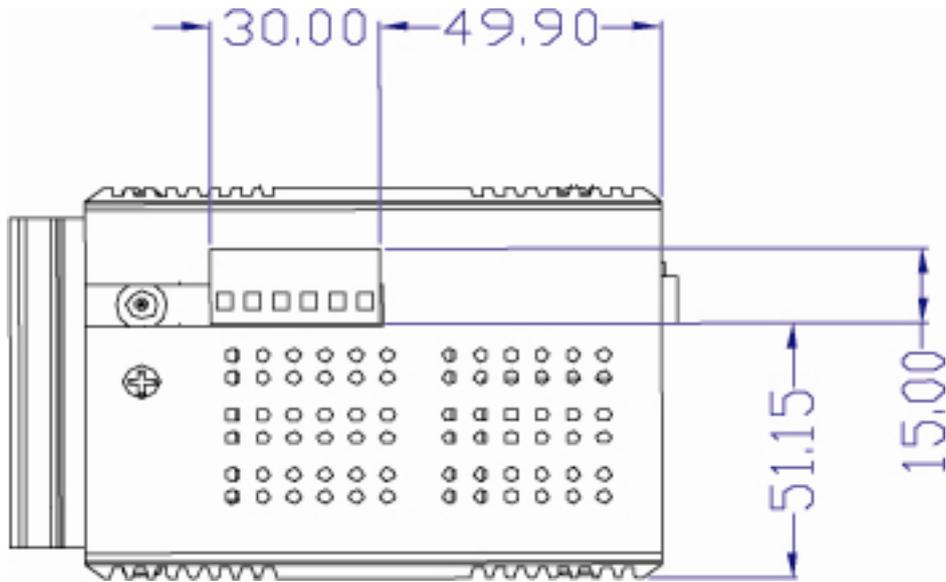
Figure 2.2-4 Top View of EKI-7554MI/SI
