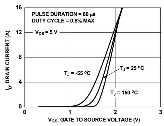
**Figure 5. Transfer Characteristics**
