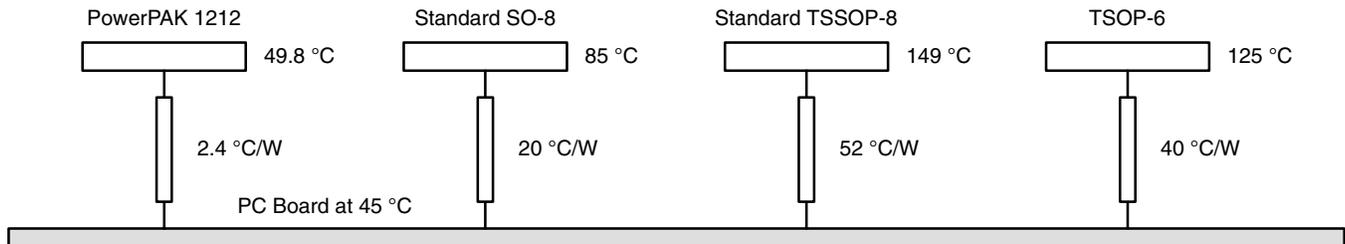
**Figure 4.** Temperature of Devices on a PC Board
