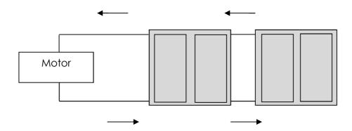
Assuming that the same amount of light is falling on both cells, wiring them in series will double the voltage supplied to motor whereas wiring them in parallel will double the current.
