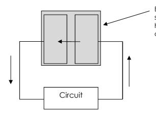
Electrons jump between two silicon layers when the sun light hits the cell. They then flow around the electric circuit.
