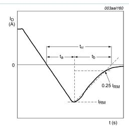
Fig. 16. Reverse recovery timing definition
