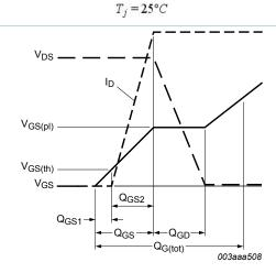
Fig. 12. Gate charge waveform definitions
