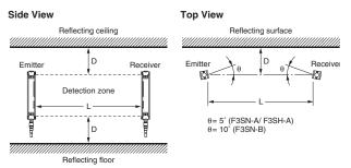
Install the F3SN-A/F3SH-A with minimum Distance D shown above from reflective surfaces (highly reflective surfaces) such as metal walls, floors, ceilings, and work pieces.
