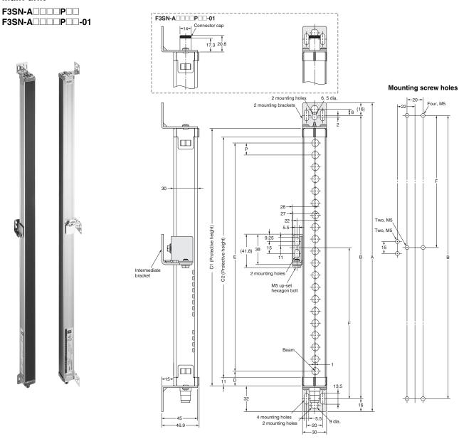
Dimensions according to the model can be calculated by using the following equations.
