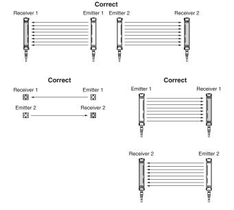
(2) Install a light interrupting wall in between sensors.
