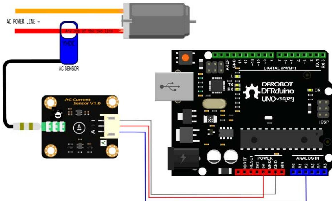
**⚠️** The probe of the AC transformer can only clamp to one AC wire at a time. It **cannot be clamped to two at the same time!**
