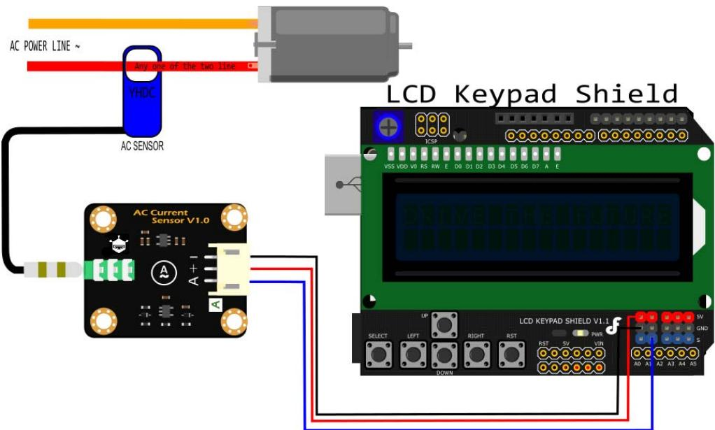
**⚠️ The probe of the AC transformer can only clamp one AC wire at a time. It cannot be clamped two at the same time!**
