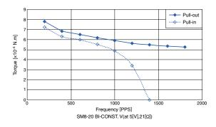
These torque values are reference only. Heat radiation conditions and temperature rise effect by duty are different on each equipment, therefore please select motors after considering the actual equipment.
