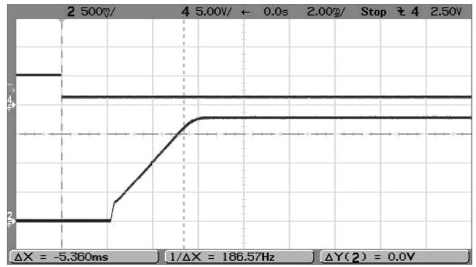
Step Load Transient Response (V<sub>in</sub>=5V, V<sub>out</sub>=1.8V, I<sub>out</sub>=6A to 3A)
