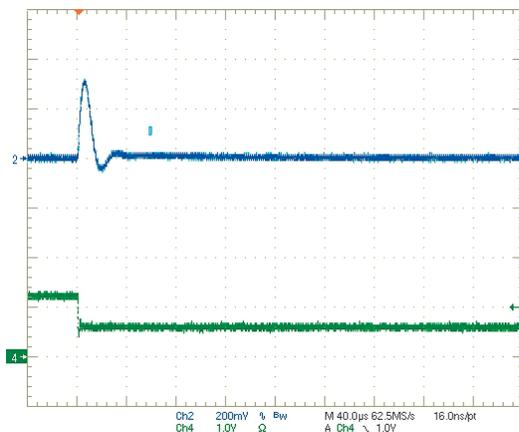
Step Load Transient Response (V<sub>in</sub>=5V, V<sub>out</sub>=1.5V, I<sub>out</sub>=3A to 6A)
