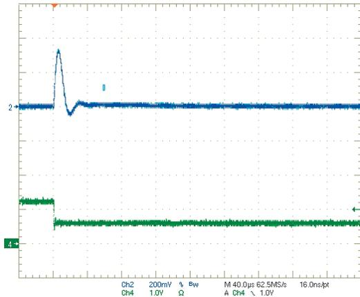
Step Load Transient Response (V<sub>in</sub>=5V, V<sub>out</sub>=1.8V, I<sub>out</sub>=3A to 6A)
