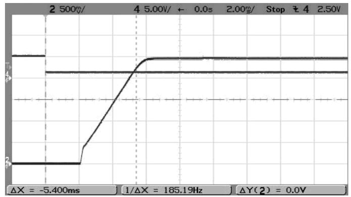
Step Load Transient Response (V<sub>in</sub>=5V, V<sub>out</sub>=2.5V, I<sub>out</sub>=6A to 3A) Trace 2=Vout, 200 mV/div. Trace 4=Iout, 5A/div.
