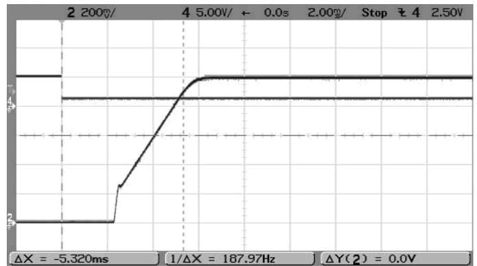
Step Load Transient Response (V<sub>in</sub>=5V, V<sub>out</sub>=1.0V, I<sub>out</sub>=6A to 3A)
