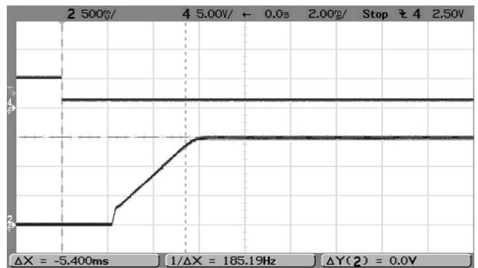
Step Load Transient Response (V<sub>in</sub>=5V, V<sub>out</sub>=1.5V, I<sub>out</sub>=6A to 3A)
