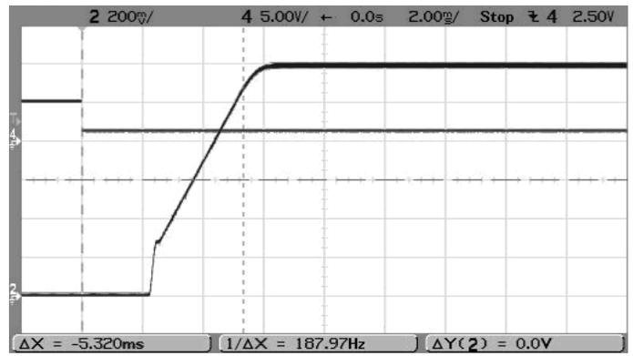
Step Load Transient Response (V<sub>in</sub>=5V, V<sub>out</sub>=1.2V, I<sub>out</sub>=6A to 3A)
