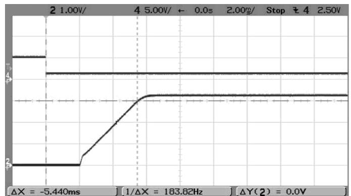
Step Load Transient Response (V<sub>in</sub>=5V, V<sub>out</sub>=3.3V, I<sub>out</sub>=6A to 3A)
