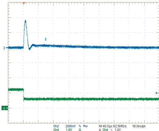
Step Load Transient Response (V<sub>in</sub>=5V, V<sub>out</sub>=3.3V, I<sub>out</sub>=3A to 6A)
