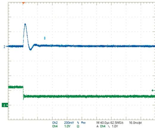
Step Load Transient Response (V<sub>in</sub>=5V, V<sub>out</sub>=1.0V, I<sub>out</sub>=3A to 6A)
