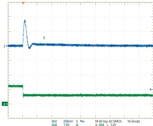
Step Load Transient Response (V<sub>in</sub>=5V, V<sub>out</sub>=2.5V, I<sub>out</sub>=3A to 6A) Trace 2=Vout, 200 mV/div. Trace 4=Iout, 5A/div.
