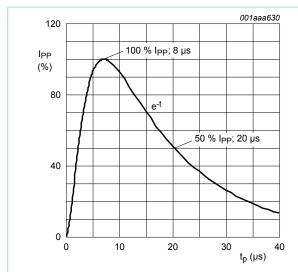
Fig. 1. 8/20 µs pulse waveform according to IEC 61000-4-5
