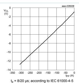
Fig. 9. Negative clamping voltage (8/20 μs pulse); typical values
