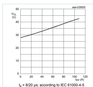
Fig. 8. Positive clamping voltage (8/20 μs pulse); typical values
