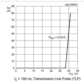
Fig. 10. Dynamic resistance with positive clamping voltage; typical value
