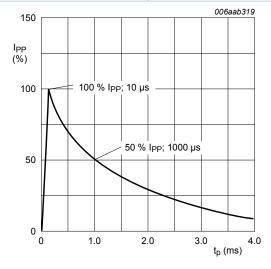
Fig. 3. 10/1000 µs pulse waveform according to IEC 61643-321
