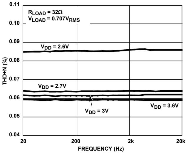
FIGURE 8. THD+N vs SUPPLY VOLTAGE vs FREQUENCY
