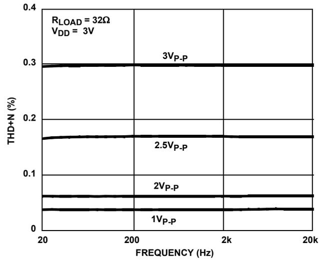
FIGURE 9. THD+N vs SIGNAL LEVELS vs FREQUENCY
