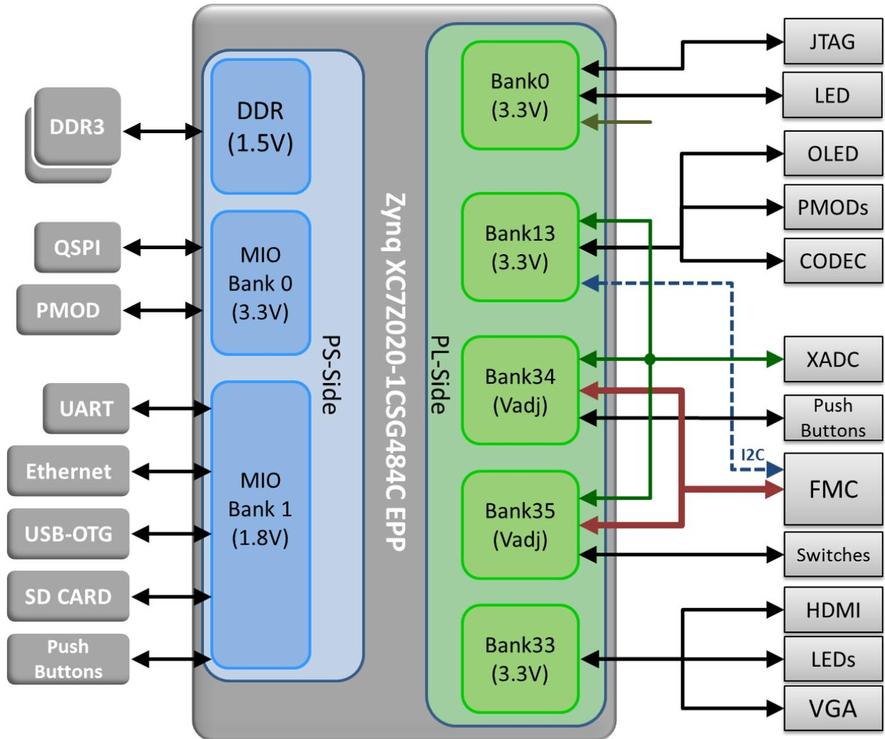
Figure 2 - Zynq Z7020 CSG484 Bank Assignments
