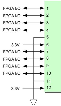
Figure 12 - Pmod Connections
