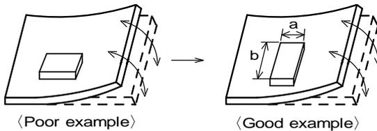
Products shall be located in the sideways direction (Length:a<b) to the mechanical stress.
