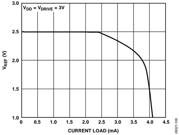
Figure 9.  $V_{REF}$  vs. Reference Output Current Drive
