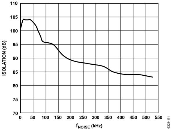
Figure 11. Channel-to-Channel Isolation,  $f_{IN} = 50$  kHz
