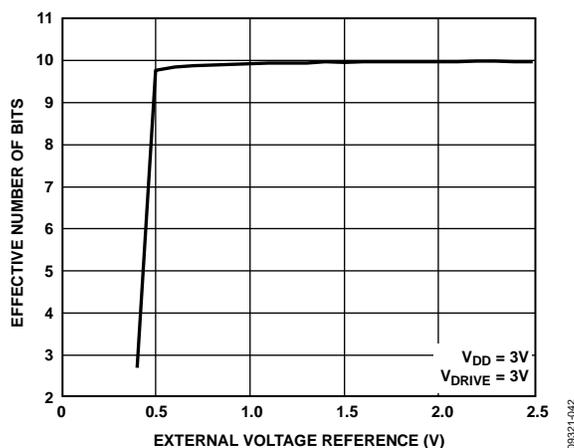
Figure 8. Effective Number of Bits vs.  $V_{REF}$
