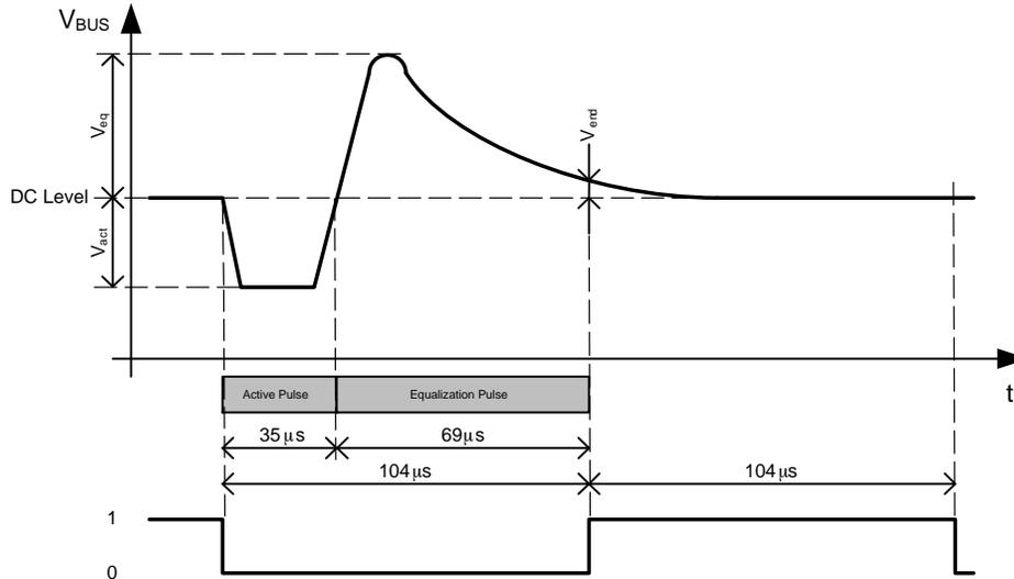
**Figure 10. KNX Bus Voltage versus Digital Value**
