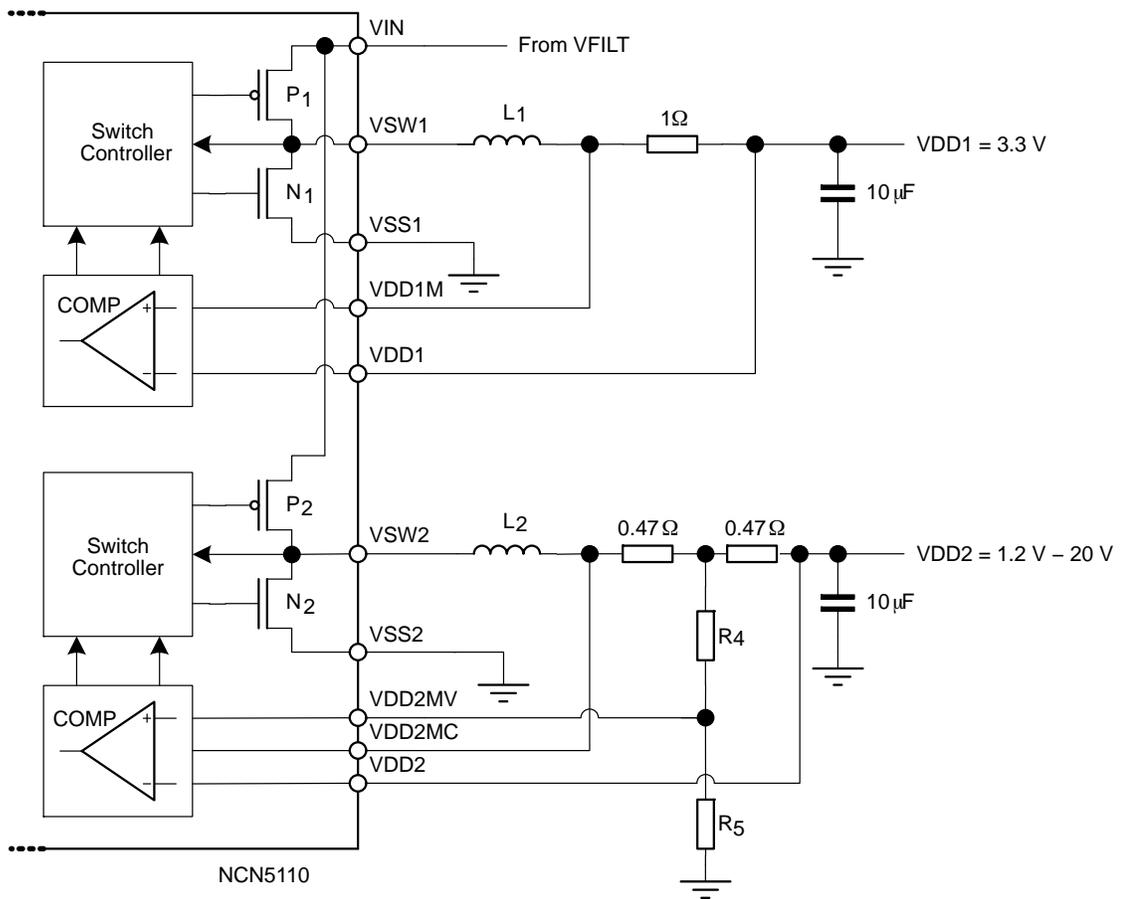
Figure 12. Fixed (VDD1) and Adjustable (VDD2) DC-DC Converter
