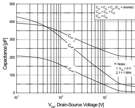
Figure 5. Capacitance Characteristics
