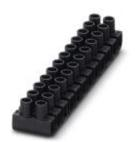
Polypropylene Europe terminal strip, black, for connecting solid conductors and stranded conductors with and without ferrules with a cross section of 0.5 to  $4~\text{mm}^2$
