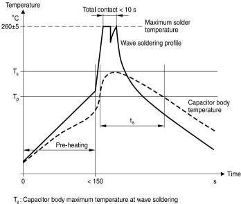
T<sub>n</sub>: Capacitor body maximum temperature at pre-heating
