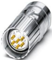
Cable connector, straight, shielded: yes, Screw locking, M23, Number of positions: 8+1, Type of contact: Male connector, Crimp connection, Cable diameter: 10 mm ... 14.5 mm
