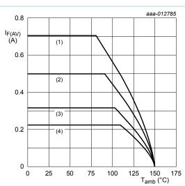
FR4 PCB, mounting pad for anode and cathode 1  $\mbox{cm}^2$  each
