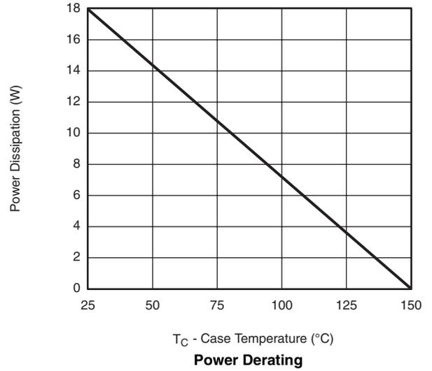
\* The power dissipation  $P_D$  is based on  $T_{J(\text{max})} = 150\text{ }^\circ\text{C}$ , using junction-to-case thermal resistance, and is more useful in settling the upper dissipation limit for cases where additional heatsinking is used. It is used to determine the current rating, when this rating falls below the package limit.
