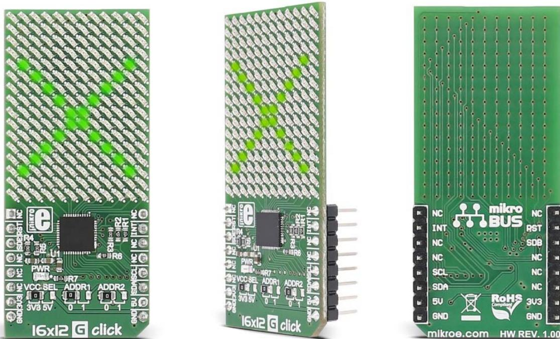
16x12 G click carries a 16x12 LED display and the IS31FL3733 matrix driver. The click is designed to run on either 3.3V or 5V power supply. It communicates with the target microcontroller over I2C interface, and the following pins on the mikroBUS™ line: INT, RST, CS.
