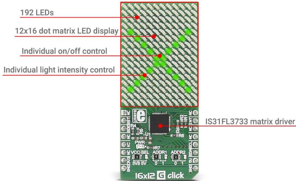
The IS31FL3733 is a general purpose 12×16 LEDs matrix driver with 1/12 cycle rate.
