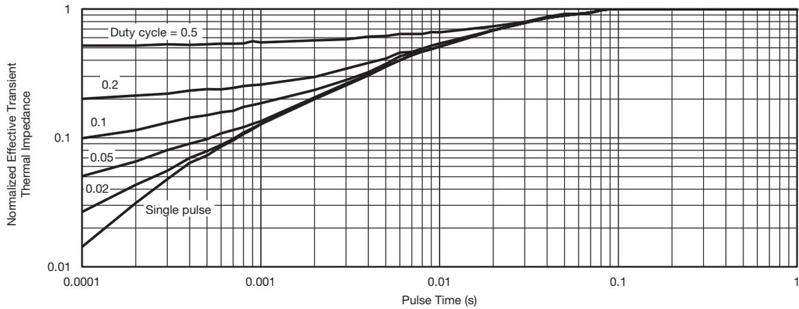
Fig. 12 - Normalized Thermal Transient Impedance, Junction-to-Case
