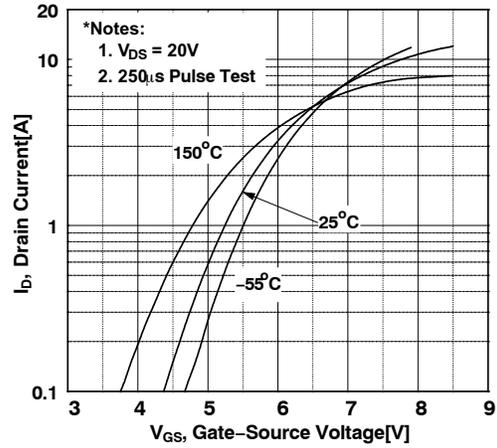
Figure 2. Transfer Characteristics
