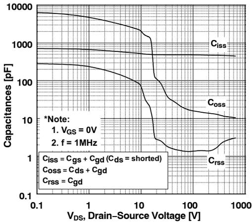
Figure 5. Capacitance Characteristics
