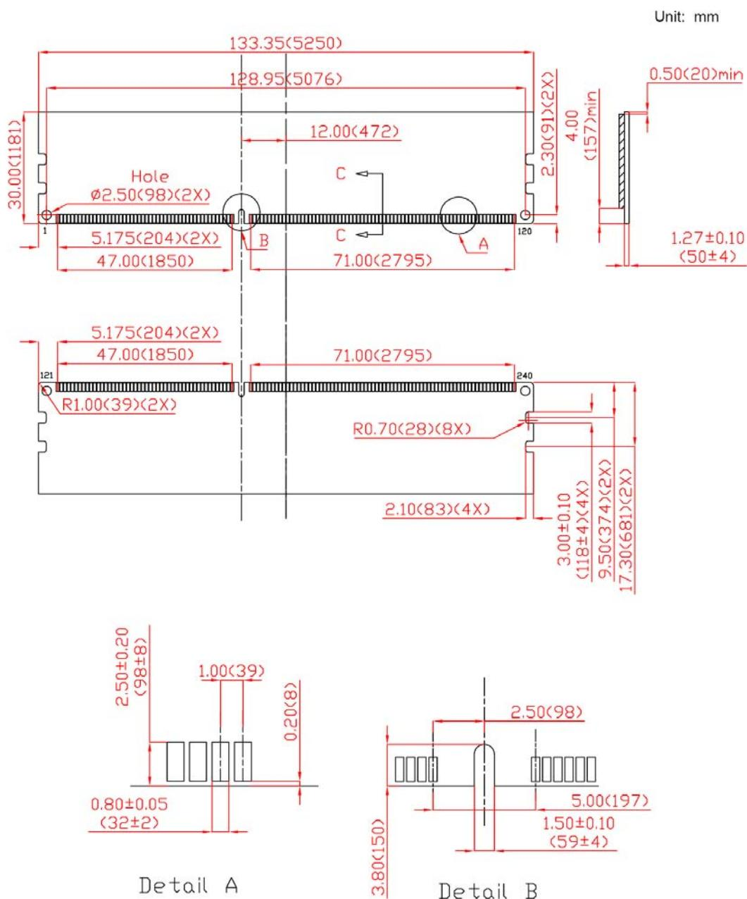
(All dimensions are in millimeters with ±0.15mm tolerance unless specified otherwise.)
