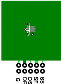
a.  $53\text{ }^\circ\text{C/W}$  when mounted on a  $1\text{ in}^2$  pad of 2 oz copper
