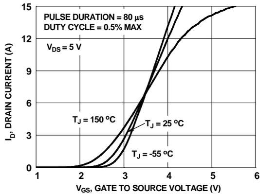
Figure 5. Transfer Characteristics
