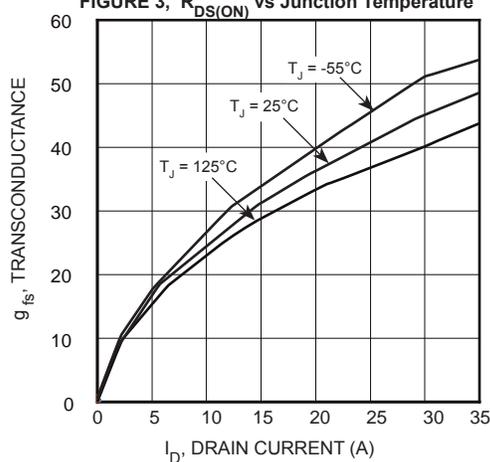
FIGURE 5, Gain vs Drain Current
