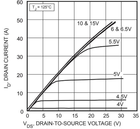
FIGURE 2, Output Characteristics
