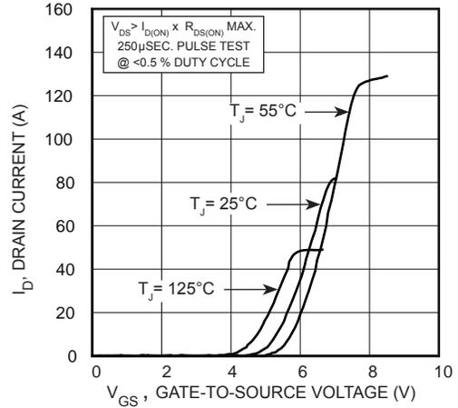
FIGURE 4, Transfer Characteristics
