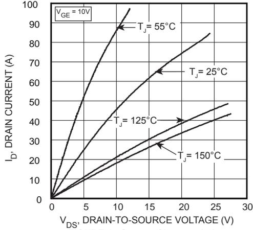
FIGURE 1, Output Characteristics
