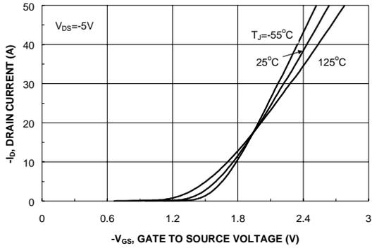
Figure 5. Transfer Characteristics.
