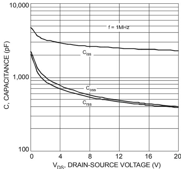
Fig. 5 Typical Capacitance
