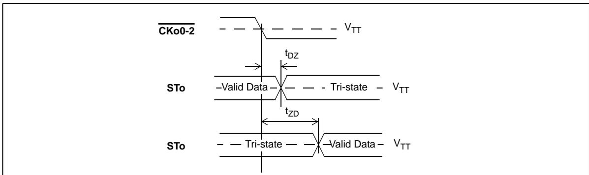
**Figure 46 - Serial Output and External Control**
