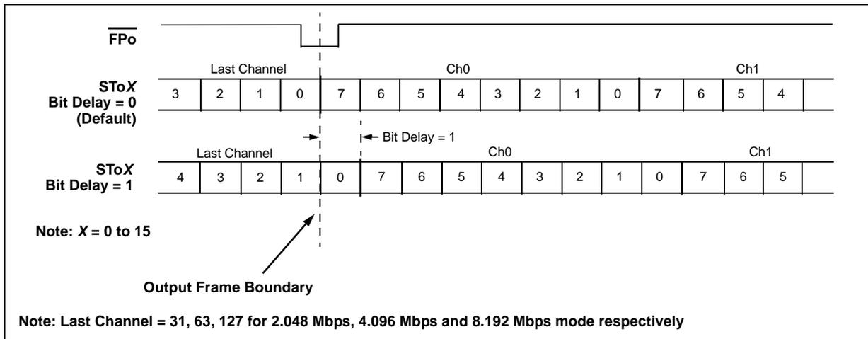
Figure 18 - Output Bit Delay Timing Diagram
