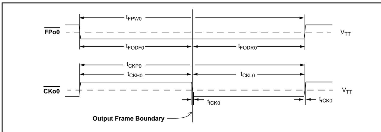
**Figure 41 -  $\overline{\text{FPo0}}$  and  $\overline{\text{CKo0}}$  Timing Diagram**
