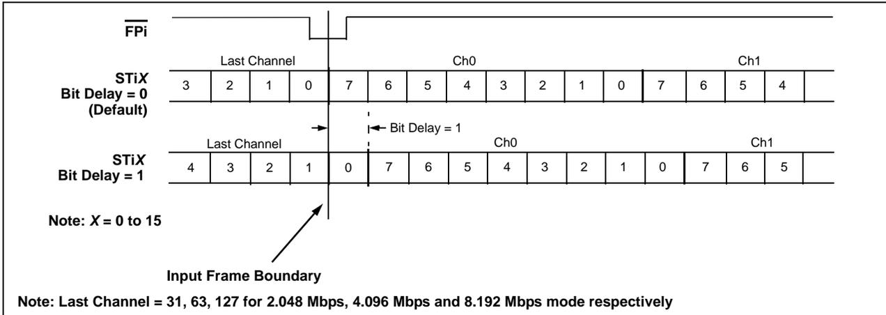
Figure 16 - Input Bit Delay Timing Diagram
