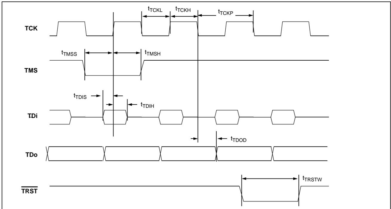
**Figure 49 - JTAG Test Port Timing Diagram**
