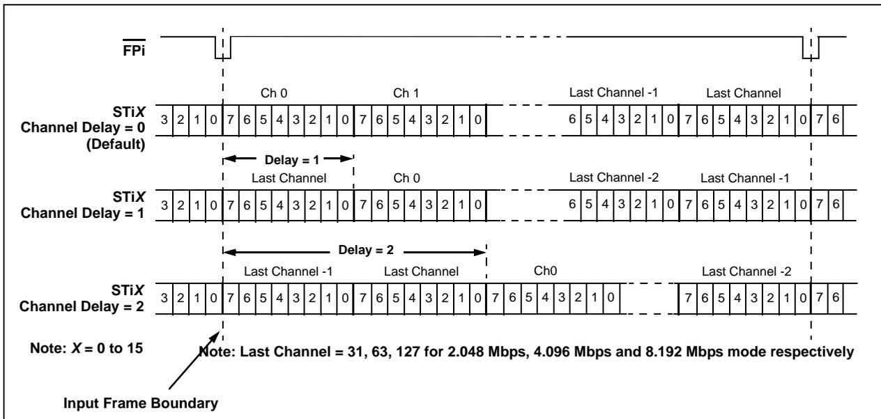
Figure 15 - Input Channel Delay Timing Diagram
