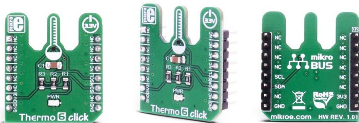
**Thermo 6 click** is a precise and versatile ambient temperature measurement click board™, based on the Maxim Integrated MAX31875 temperature sensor. This sensor has a great combination of features, such as wide range of temperature measurement, excellent measuring accuracy, and small die size, coupled with the very low power consumption - attributes that make this sensor a great choice for many different applications.
