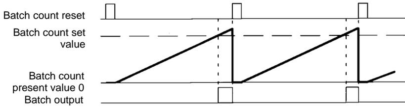
The batch count output holds until reset by the batch count reset. The present value of the batch count advances continuously.
