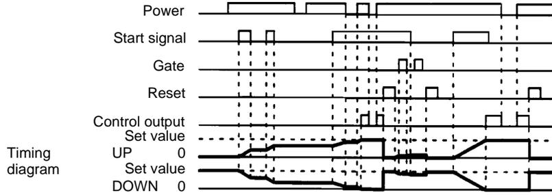
Timing begins on the leading edge of the start signal. The control output is energized when the cumulative elapsed time of the start signal is equal to the preset time. The output is sustained until power is interrupted or a reset signal is applied.
