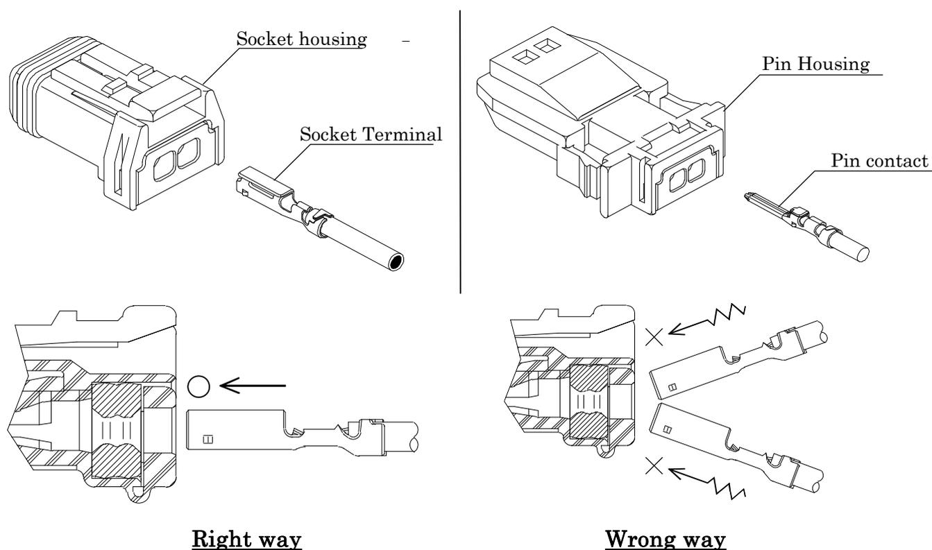
Fig.4-1 Contact insertion
