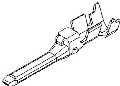
Fig.2-3 Pin contact.
