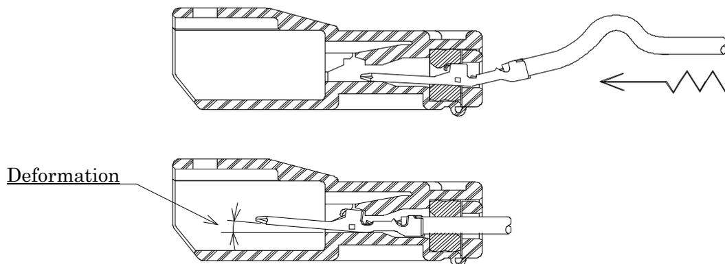
Fig.4-2 Example, contact deformation by wrong contact insertion.
