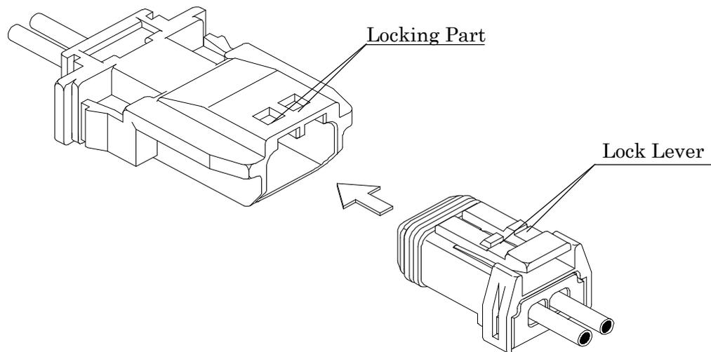
Fig.6-1 Connector insertion
