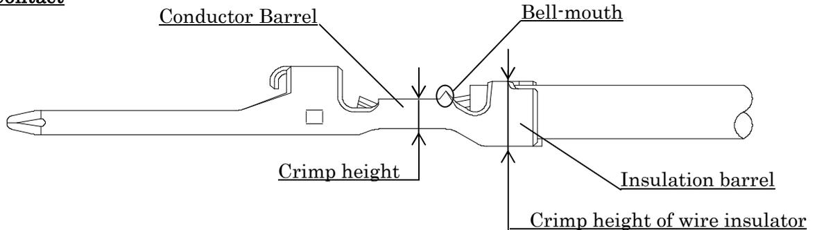
Fig.3-3 Part description of pin contact
