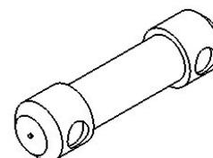
Fig.2-5 Dummy plug.
