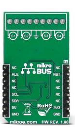
**PAC1934 click** carries the PAC1934 four channel DC power/energy monitor from Microchip. The click is designed to run on either 3.3V or 5V power supply. It communicates with the target microcontroller over an I2C interface.
