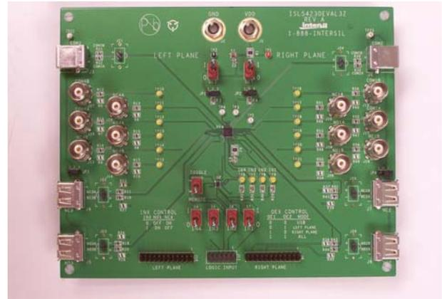
FIGURE 1. ISL54230EVAL2Z, ISL54230EVAL3Z EVALUATION BOARD
