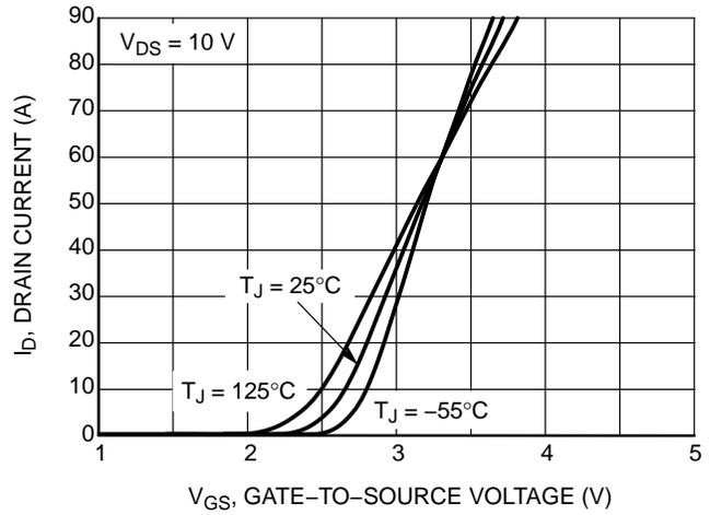
Figure 2. Transfer Characteristics
