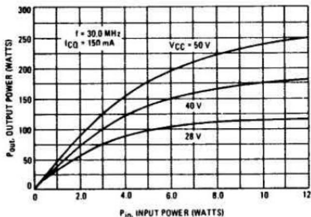
FIGURE 3 — OUTPUT POWER versus SUPPLY VOLTAGE
