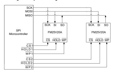
Figure 2. System Configuration with SPI Port
