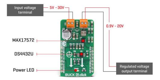
The MAX17572 features a robust overload and short circuit protection. When the internally set current limit of 1.7A is exceeded, the high side MOSFET is turned off and the hiccup mode is triggered. This mode suspends the operation for 32,768 duty cycles after which the soft start sequence is reattempted. If the faulty condition is still present and the feedback voltage remains under 0.58V, the switching frequency will be halved to avoid overheating during the restart sequence.
