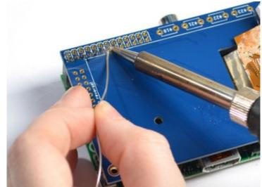
Heat up your soldering iron, and grab some solder. Start by tack-soldering one of the corners while pressing on the plate to make it sit flat. Once you have one or two pins done you can continue to solder each of the pins.
