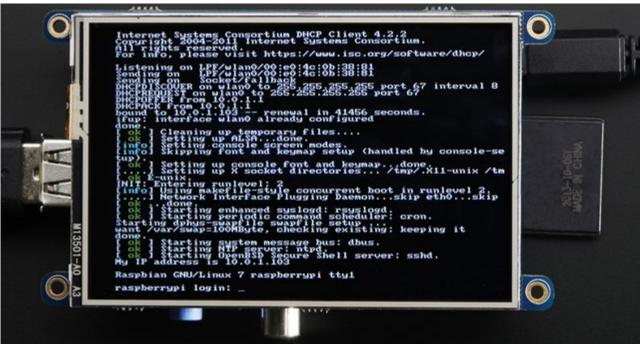
One fun thing you can do with the display is have it as your main console instead of the HDMI/TV output. Even though it is small, with a good font you can get 20 x 40 of text. For more details, check out <a href="https://github.com/notro/fbtft/wiki/Boot-console">https://github.com/notro/fbtft/wiki/Boot-console</a> (http://adafru.it/cXQ)
