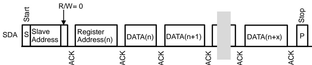
Figure 12.7. WRITE Operation
