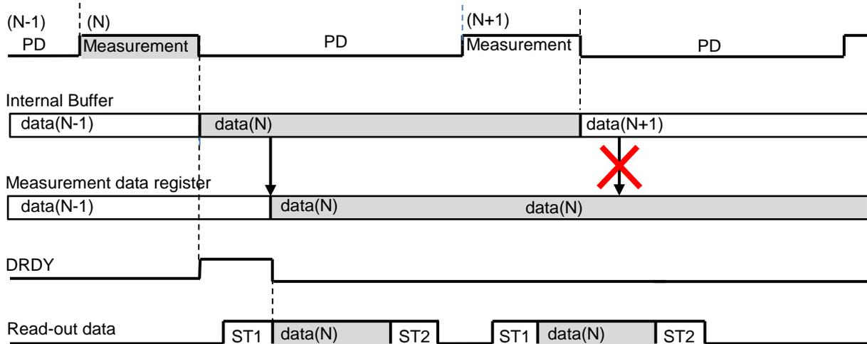
Figure 11.7. Read-out data within a measurement period
