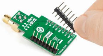
Turn the board upside down so that the bottom side is facing you upwards. Place shorter pins of the header into the appropriate soldering pads.
