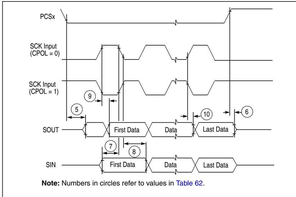
Figure 45. DSPI modified transfer format timing — slave, CPHA = 1
