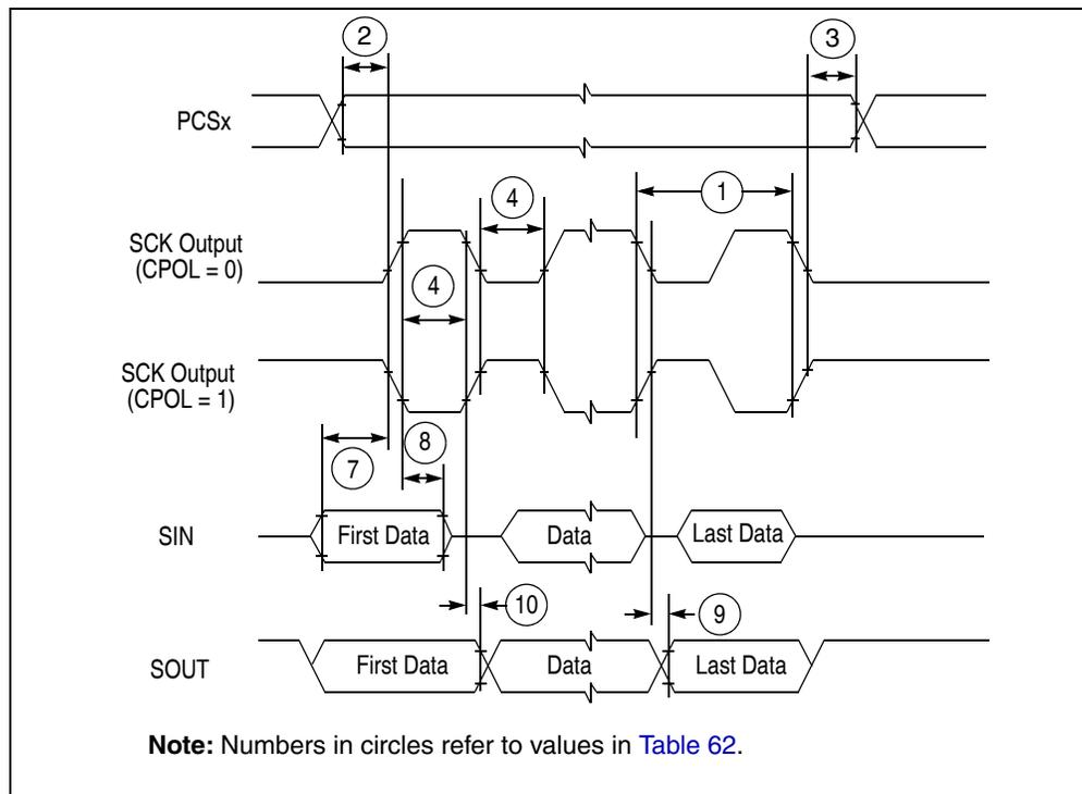
Figure 38. DSPI classic SPI timing — master, CPHA = 0
