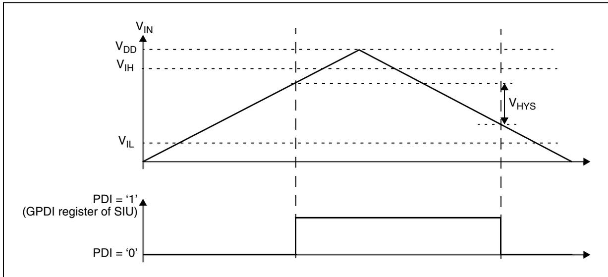
Figure 14. I/O input DC electrical characteristics definition
