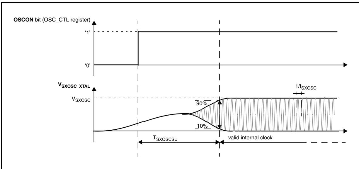
Figure 20. Slow external crystal oscillator (32 KHz) timing
