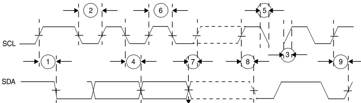
**Figure 46. I<sup>2</sup>C input/output timing**
