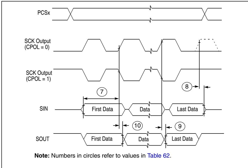
Figure 43. DSPI modified transfer format timing — master, CPHA = 1
