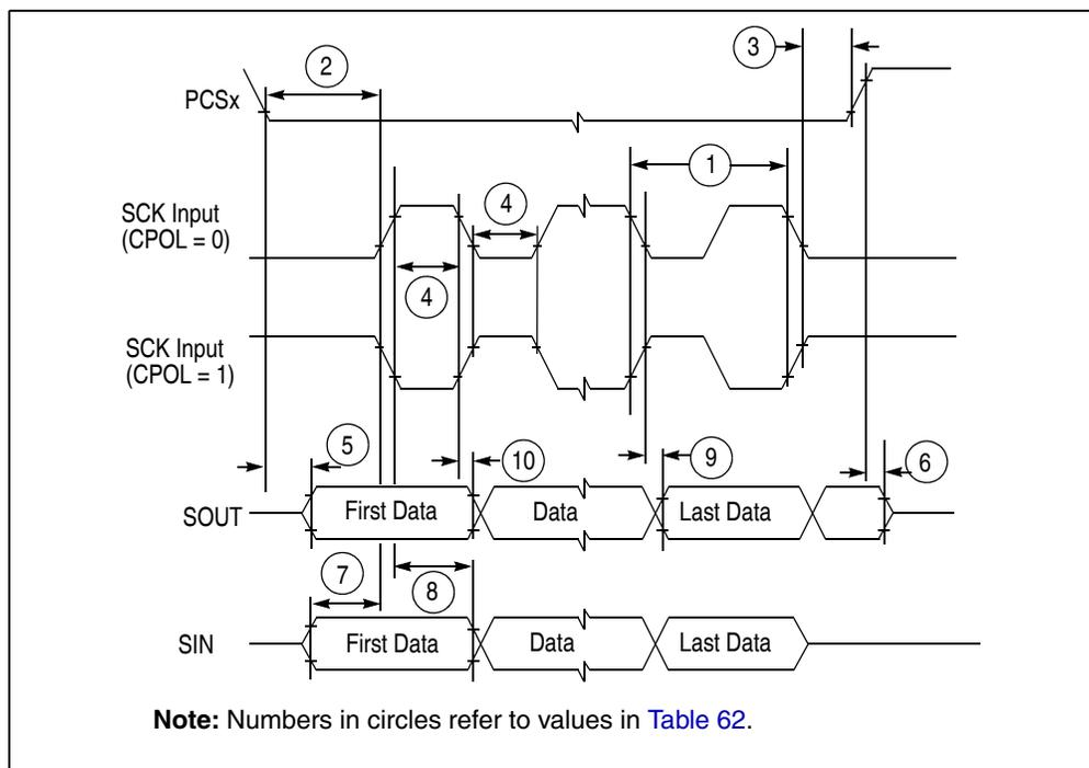
Figure 40. DSPI classic SPI timing — slave, CPHA = 0
