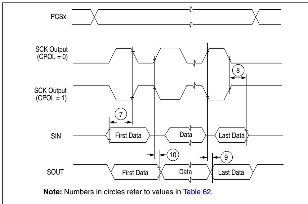
Figure 39. DSPI classic SPI timing — master, CPHA = 1
