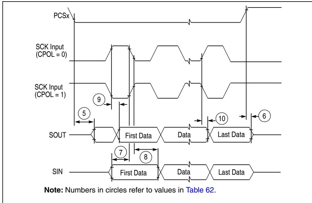
**Figure 41. DSPI classic SPI timing — slave, CPHA = 1**
