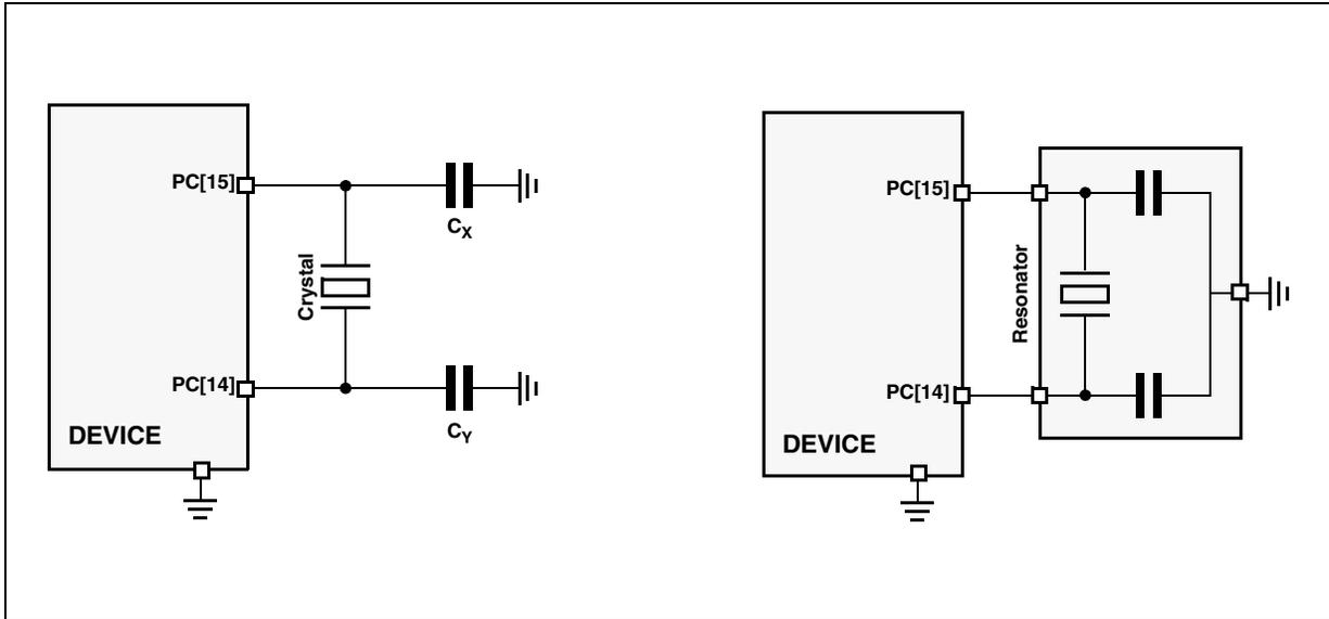
Figure 19. Crystal oscillator and resonator connection scheme
