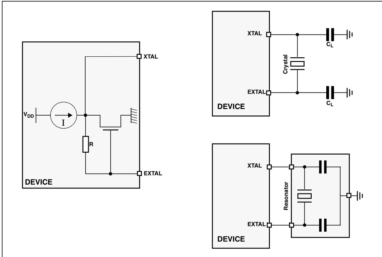
Figure 17. Crystal oscillator and resonator connection scheme
