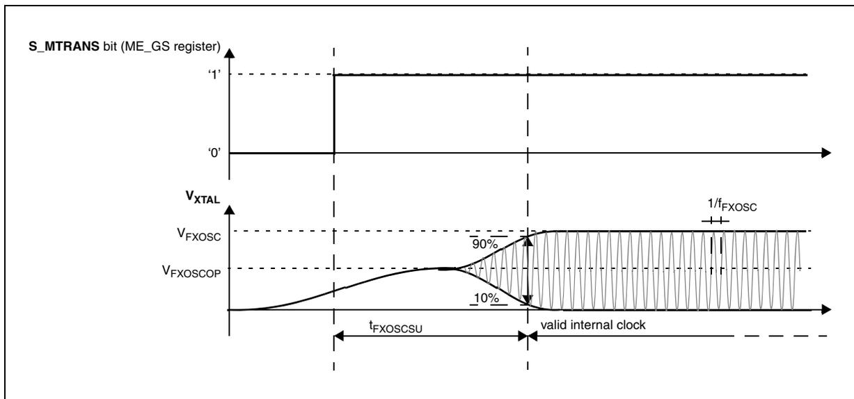
**Figure 18. Fast external crystal oscillator (4–16 MHz) electrical characteristics**
