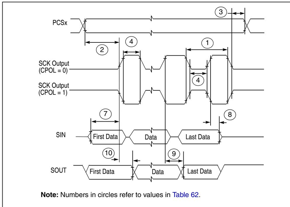
**Figure 42. DSPI modified transfer format timing — master, CPHA = 0**
