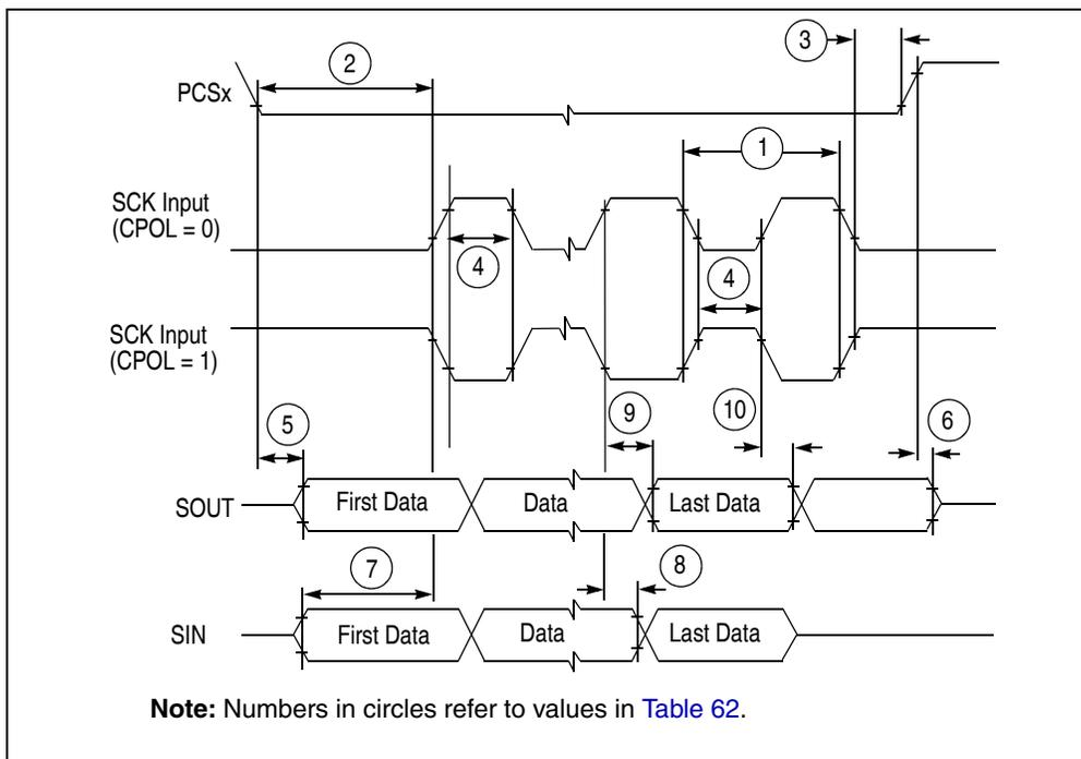
Figure 44. DSPI modified transfer format timing — slave, CPHA = 0
