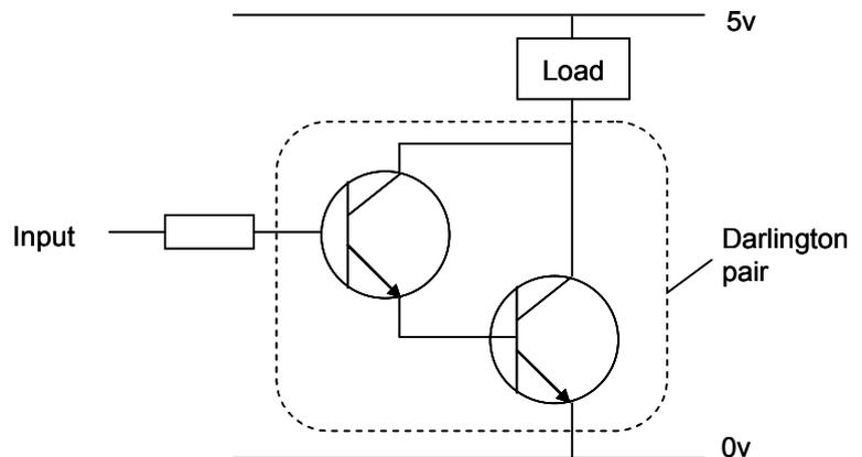
The current gain varies for different transistor and can be looked up in the datasheet for the device. Typically, it may be 100. This would mean that the current available to drive the load would be 100 times larger than the input to the transistor.
