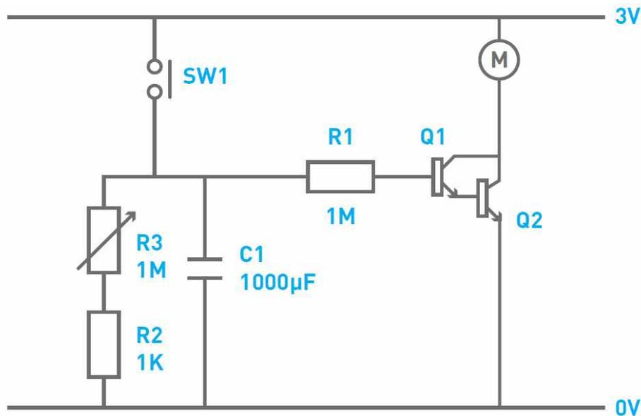
When the switch (SW1) is pressed the capacitor (C1) charges. When the switch is released the capacitor (C1) slowly discharges through the resistors (R2 & R3). R2 is just present to make sure that the batteries aren't shorted if the switch is pressed and the variable resistor R3 is set to zero.
