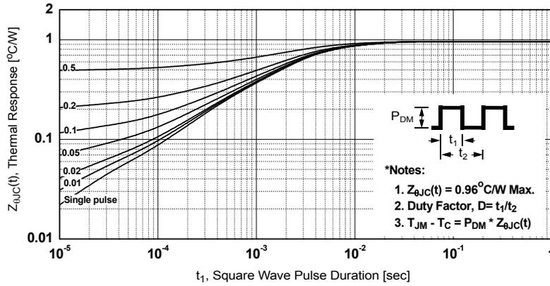
Figure 14. Transient Thermal Response Curve - FDPF8N50NZ
