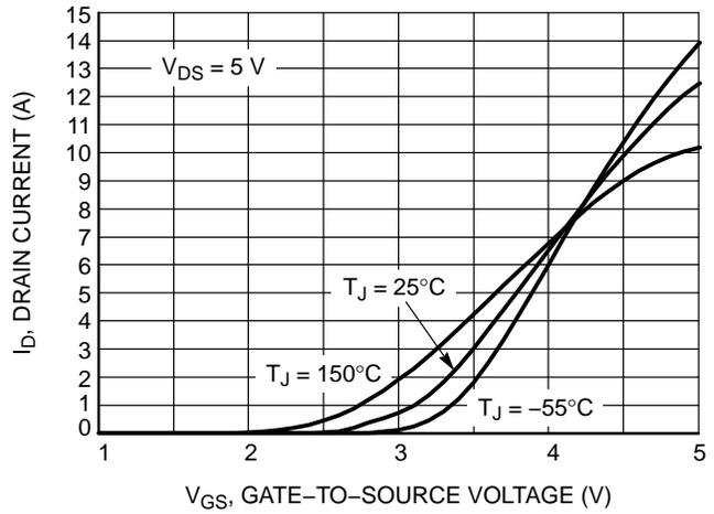
Figure 2. Transfer Characteristics
