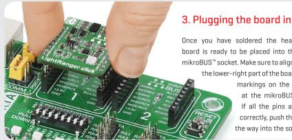
Once you have soldered the headers your board is ready to be placed into the desired mikroBUS™ socket. Make sure to align the cut in the lower-right part of the board with the
