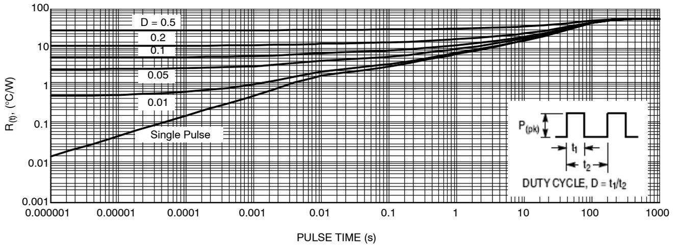
Figure 10. PCB Cu Area 650 mm<sup>2</sup> PCB Cu thk 1 oz Power (J1) 0.800 W Power (J2) 0.800 W
