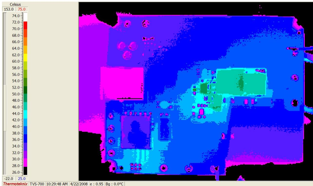
Figure 8. Temp Data (37Vport, 5A, Bottom)
